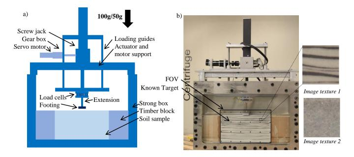
Figure 1. a) Schematic of the actuator and strongbox assembly, b) a general view of set-up and image analysis parameters.
