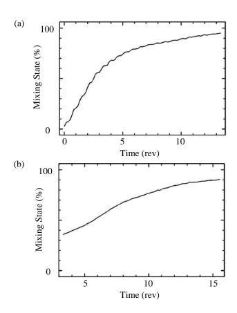
Figure 7. The mixing state for a high shear mixer with a blade impeller as a function of time for: (a) azimuthal and (b) radial mixing from DEM simulations by Cleary and Sinnott (2008).
