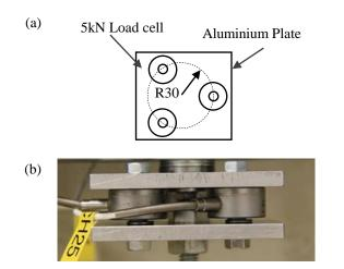
Figure 2. Force plate for measuring axial reaction load, a) plan and b) general view.
