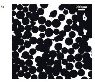
Figure 10. a) Direct shear results for dyed and non-dyed glass ballotini, b) dyed glass Ballotini viewed under a microscope.
