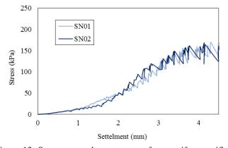
Figure 13. Stress vs. settlement curves for centrifuge verification tests.
