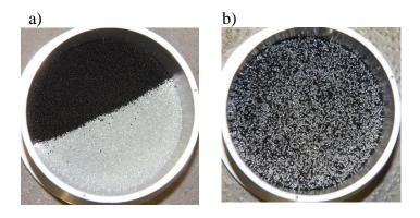
Figure 8. Mixing of dyed and non-dyed glass ballotini, a) initial state, b) mixing state after 60 sec.
