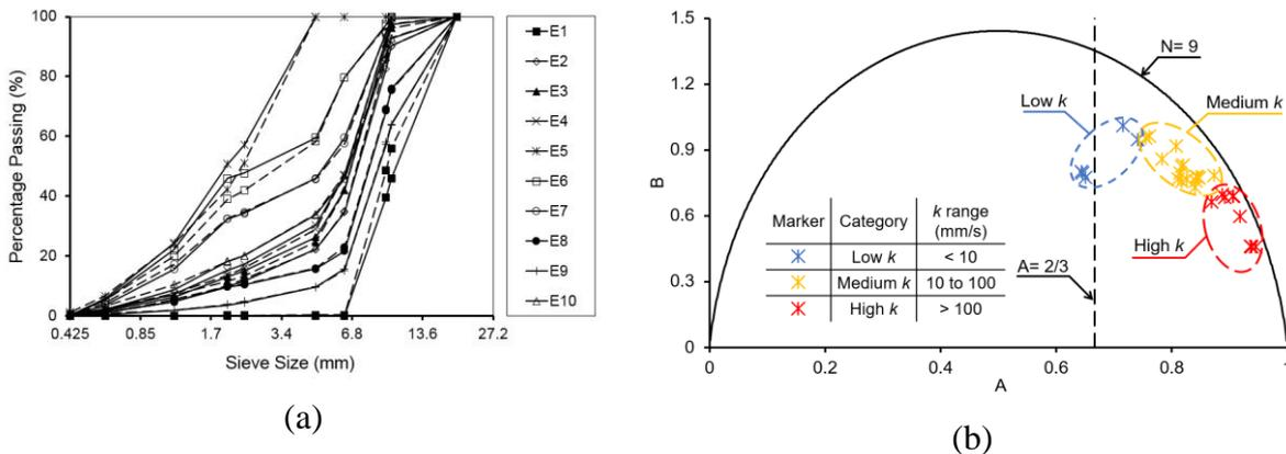
Figure 5. (a) Grading curve set out of three tested sets with varying fine content. (b) Permeability variation in normalized diagram [11].
