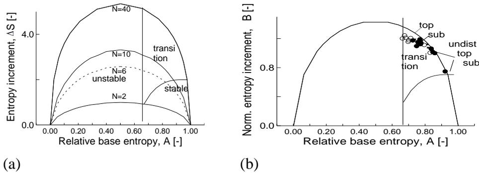
Figure 3. (a) Internal or grain structure stability criterion in the non-normalized diagram. (b) Internal or grain structure stability criterion in the  $N=17$  related normalized diagram, with the indication of the degradation example of waste rock in open pit mine rehabilitation (the topsoil samples are more degraded [10]).
