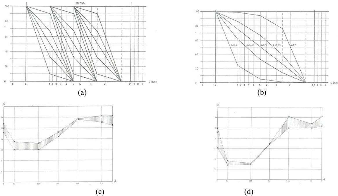
Figure 6. The relation of critical state friction angle and the entropy coordinate  $A$  in case of optimal sand soil mixtures ([15]). (a) and (b) grading curves of the 2- and 4-fraction sand mixtures. (c) and (d) critical state friction angle of the 2- and 4-fraction sand mixtures as  $A$  varies between 0 and 1.
