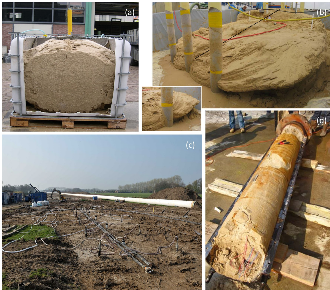
Fig. 16 MICP trials in three scales: a cubic metre sand box [103]—photograph from [117]; b 100 cubic metre sand box [109]; c 1000 cubic metre field-scale mediation [103]; d MICP at large scale: MICP-treated 400-mm dia. column by Soletanche-Bachy [118]
